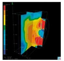
FIGURE 2: A principle sketch of the radiator package on a rock-drill machine and the velocity profile over the radiator surface
