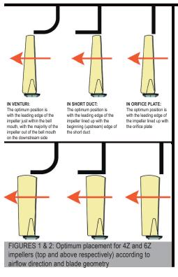
through more than 90°. There are, however, occasions when the turbulent flow produced in non-ideal conditions can result in a more even flow through the entire surface area of a radiator, resulting in better cooling.
